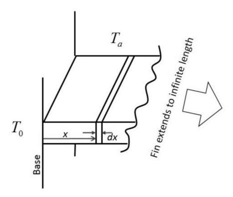
The steady state one dimensional energy balance on an element of the fin of thickness dx at a distance x from its base yields
