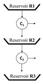
The efficiencies of the engines C<sub>1</sub> and C<sub>2</sub> are 0.40 and 0.35, respectively. If the temperature of Reservoir R1 is 800 K, then the temperature (in K) of Reservoir R3 is \_\_\_\_\_ (round off to nearest integer).
