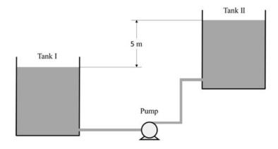
Both the tanks are open to the atmosphere. The total frictional head loss for the pipe system is 1.0 m of water.
