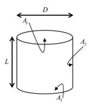
$F_{ij}$  denotes the fraction of radiation energy leaving the surface  $A_i$  which reaches the surface  $A_j$ . It is also known that  $F_{13}=3-2\sqrt{2}$ . Which one of the following is correct?
