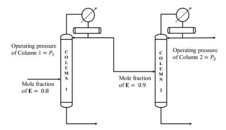
Mole fraction of  $\mathbf{E}$  in the distillate obtained from column 1 is 0.9. If the column pressures  $P_1$  and  $P_2$  are in kPa, which one of the following is correct?
